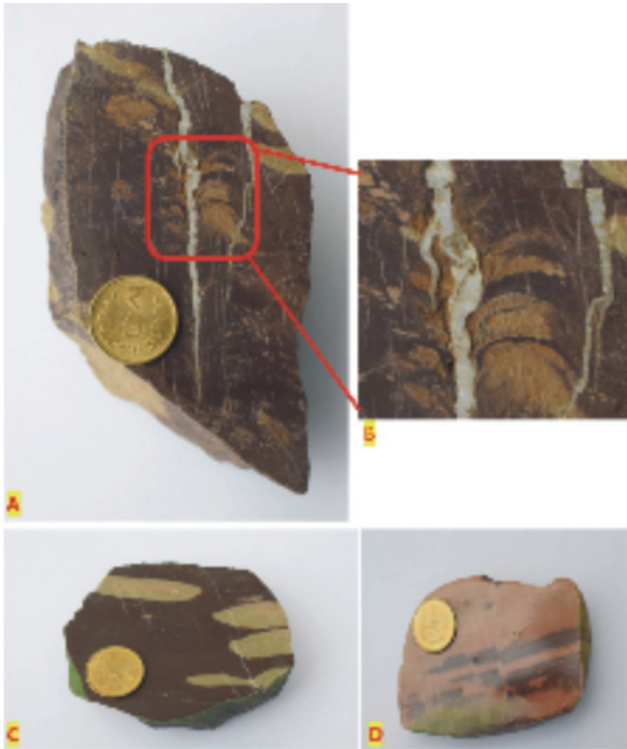
Plate 2: A. Polished slab showing columnar stromatolite column B. Close-up view of A with clearly visible dark and light lamination C. Compressed calcareous nodules in chocolate coloured shales D. Microfracturing in carbonate layers (Scale- Coin of 5 Rupees)
